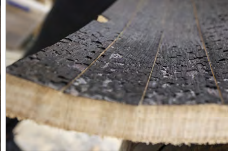
Steve West uses screws to add structure to the whiskey barrel so that it maintains its integrity throughout the process. The screws also add an ornamental finish to the barrel. Photo by Andrea Schlepphorst. | One of the final steps in transforming a whiskey barrel into fine furniture is to scrape the charred insides of the barrel, then apply three coats of sealant to the staves to preserve the grains, and give the finished barrel a rich tone. Photo by Cindy Price
