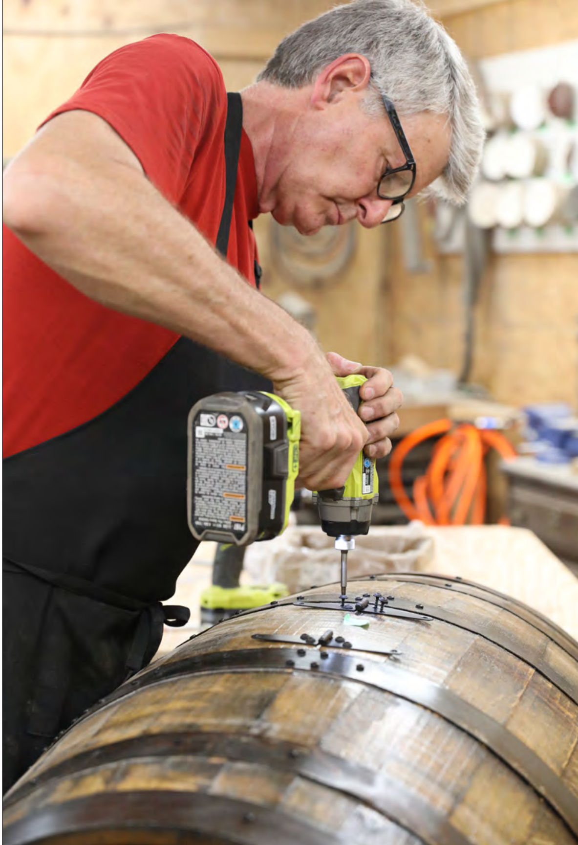
Steve West uses screws to add structure to the whiskey barrel so that it maintains its integrity throughout the process. The screws also add an ornamental finish to the barrel. Photo by Andrea Schlepphorst. | One of the final steps in transforming a whiskey barrel into fine furniture is to scrape the charred insides of the barrel, then apply three coats of sealant to the staves to preserve the grains, and give the finished barrel a rich tone. Photo by Cindy Price
